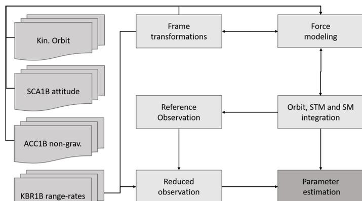
Fig. 1: Simplified gravity field recovery procedure.
