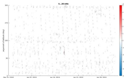
Fig. 5: LRI range rate post-fit residuals as Time/Argument of Latitude (TAL) diagram. Values above  $3\sigma$ . For Jan. 2019
